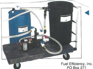
The "Pump Cart System" is a complete mobile pumping package. This unit starts on a 2' by 4' Rubbermaid ® heavy-duty plastic cart with 5" swivel wheels. A 30 gallon circulation drum with a valved drain is secured to the cart's steel handle. The pump is mounted directly to the cart with all the necessary valves and hoses. The pump is also GFCI wired and switched in a mounted weather-proof electrical box with a 20'cord. This unit comes completely assembled and packed on a skid ready for use.
